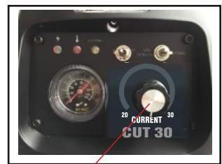
(6) Set the amperage dial and ensure switch is in Cutting mode
