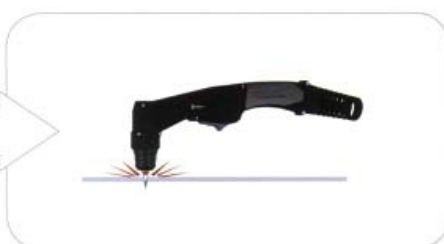
If sparks are spraying up from the work piece, you are moving the torch too fast, or you don't have enough amps set.
