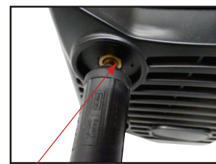
(2) Connect the earth lead to the output terminal of the machine and tighten.
