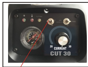
(5) select 2T or 4T torch control .2T is standard manual operation mode
