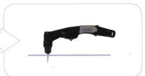
Hold the torch vertical and watch the arc as it cuts along the line.
