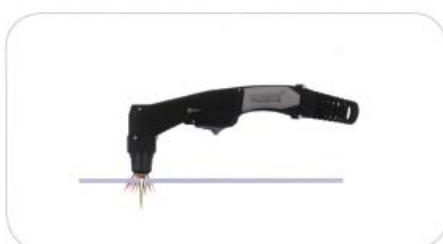
When cutting make sure that sparks are exiting from the bottom of the work piece.
