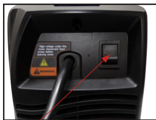
(4) Connect the machine to the correct power supply and switch on the machine using the on/off switch located at the rear of the machine..
