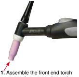
1. Assemble the front end torch parts use the correct size and type of tungsten electrode for the job, the tungsten electrode requires a sharpened point for DC welding
