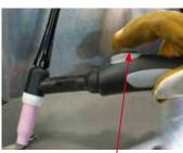
6. Release the torch switch to bring in the end of the welding sequence dependant of 2T or 4T trigger function choice
