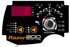
Set the AC Balance by pressing the encoder to cycle through to illuminate the AC Balance icon. Set the AC Balance by turning the encoder knob. The set AC balance will appear in the digital display
