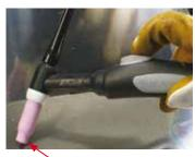
4. Lay the outside edge of the Gas Cup on the work piece with the Tungsten Electrode 1- 3mm from the work piece
