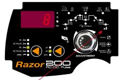
Set the post gas time by pressing the encoder to cycle through to illuminate the Post Gas
