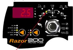
Set the Up Slope by pressing the encoder to cycle through to illuminate the Up Slope icon. Set the up slope time by turning the encoder knob. The set up slope time will appear in the digital display
