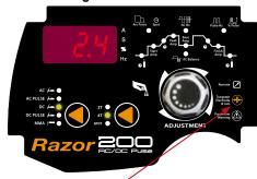
(2) Select the tungsten diameter required by pushing the encoder repeatedly, cycle through to illuminate the Tungsten Electrode icon. Set the size required by turning the encoder knob. The set size will appear in the digital display.
