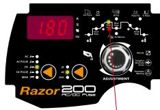
Set welding amps by pressing the encoder to cycle through to illuminate the Peak Ampicon. Set the amperage by turning the encoder knob. The set welding amperage will appear in the digital display
