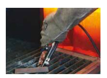
**6)** Connect the Earth Clamp securely to the work piece or the work bench.
