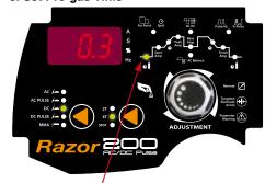
Set the pre gas time by pushing the encoder repeatedly, cycle through to illuminate the Pre Gas of icon. Set the time by turning the encoder knob. The set time will appear in the digital display
