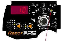
Set the finish amps by pressing the encoder to cycle through to illuminate the Finish Amps icon. Set the finish amps by turning the encoder knob. The set finish amps will appear in the digital display
