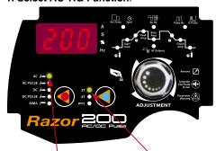
Select AC TIG by pressing the button until the AC icon illuminates. Select 2T or 4T trigger function as required by the pushing the button to cycle through the trigger options. The icon will illuminate for the selected trigger option.
