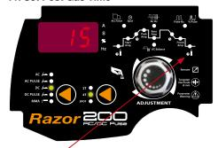
Set the post gas time by pressing the encoder to cycle through to illuminate the Post Gas (b) icon. Set the post gas time by turning the encoder knob. The set post gas time will appear in the digital display
