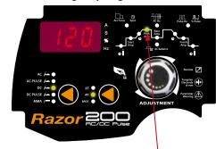
Set welding amps by pressing the encoder to cycle through to illuminate the Peak Amp icon. Set the amperage by turning the encoder knob. The set welding amperage will appear in the digital display
