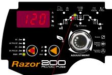
(4) Set the amperage by selecting the Peak Amp icon pressing the Encoder Knob until the Peak Amp icon illuminates. Turn the encoder knob to set the amperage according to the electrode type and size being used as recommended by the electrode manufacturer. The set amperage will show in the digital display panel.
