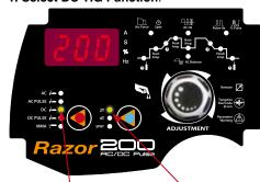
Select DC TIG by pressing the button until the DC icon illuminates. Select 2T or 4T trigger function as required by the pushing the button to cycle through the trigger options. The icon will illuminate for the selected trigger option.
