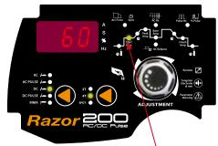
Set the Start Amps by pressing the encoder to cycle through to illuminate the Start Amp icon. Set the start amps by turning the encoder knob. The set start amps will appear in the digital display
