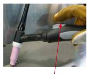
**6.** Release the torch switch to bring in the end of the welding sequence dependant of 2T or 4T trigger function choice
