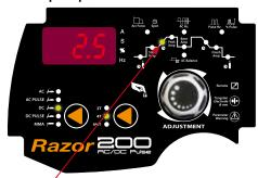
Set the Up Slope by pressing the encoder to cycle through to illuminate the Up Slope icon. Set the up slope time by turning the encoder knob. The set up slope time will appear in the digital display
