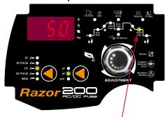
Set the finish amps by pressing the encoder to cycle through to illuminate the Finish Amps icon. Set the finish amps by turning the encoder knob. The set finish amps will appear in the digital display
