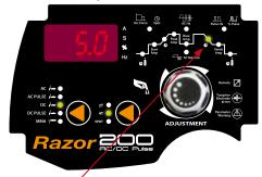
Set the down slope by pressing the encoder to cycle through to illuminate the Down Slope icon. Set the down slope time by turning the encoder knob. The set down slope time will appear in the digital display
