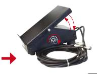
3. Activate by holding down the foot pedal for 5 seconds, the remote icon will illuminate. Up & down travel of the foot pedal will adjust the welding amperage during welding. The side potentiometer knob will allow manual set and adjustment.
