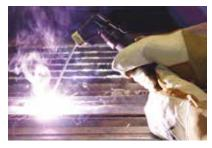
**6)** Hold the electrode slightly above the work piece to maintain the arc while travelling at an even speed to create and even weld deposition.
