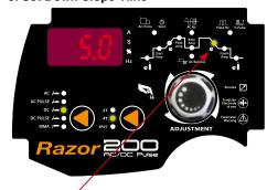
Set the down slope by pressing the encoder to cycle through to illuminate the Down Slope icon. Set the down slope time by turning the encoder knob. The set down slope time will appear in the digital display
