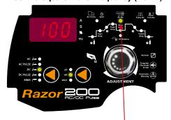
Set the AC Hz by pressing the encoder cycle through to illuminate the AC Hz icon. Set the AC Hz by turning the encoder knob. The set AC Hz will appear in the digital display
