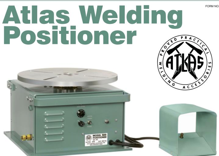
The Atlas Model 500 Welding Positioner is designed for those heavy parts turning jobs that require a truly rugged industrial piece of equipment. It will handle properly balanced loads of 500 pounds in the horizontal position.
